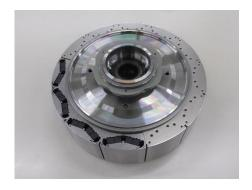
Traction motor with heavy-rare-earth-free magnets
